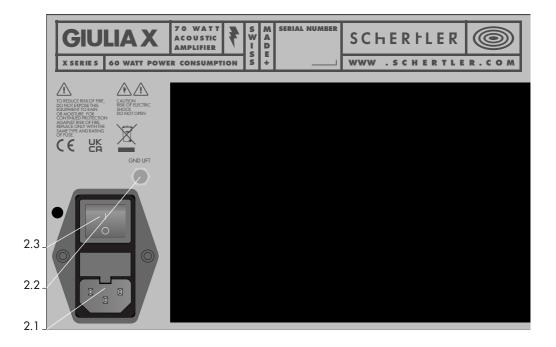
2.1. POWER ON/OFF: System ON/OFF switch.
